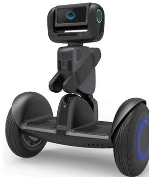
Figure 2: 2-wheeled Loomo robot.
